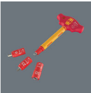
The VDE-insulated T-handle 410 i VDE A RA adapter screwdriver may only be used with the 1/4" VDE bit sockets and sockets from the Wera Zyklop VDE series 8740, 8760, 8767 and 8790.
